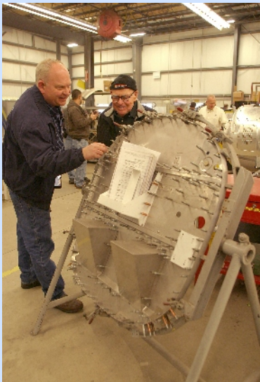
Paul and John check out the stainless steel firewall being assembled for a Great Lakes T2-A1.
