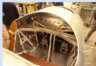
A WACO YMF-5D fuselage under construction. How sweet is that rotisserie!
