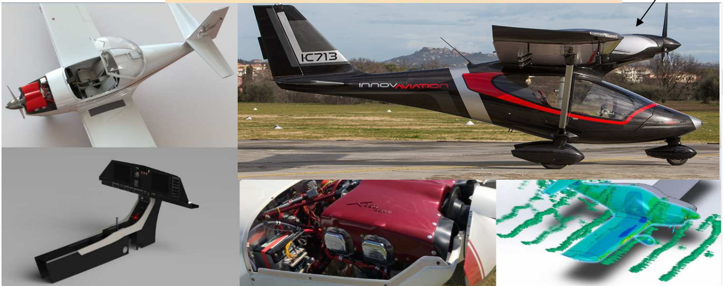
From Top Left - 3D Render of Complete Aircraft Assembly with Cowl Open, Finite Element Analysis (FEA) of Main Spar, 3D Render of Complete Aircraft Assembly with Wing Exposed, Computer Aided Optimization of Avionics Panel and Center Console, Engine Cooling Plenum, Surface Plot with Overlaid Flow Trajectories
