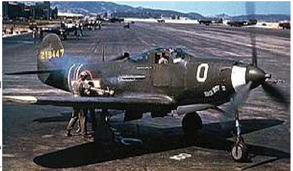
Bell XP-39 showing the position of the supercharger air intake
