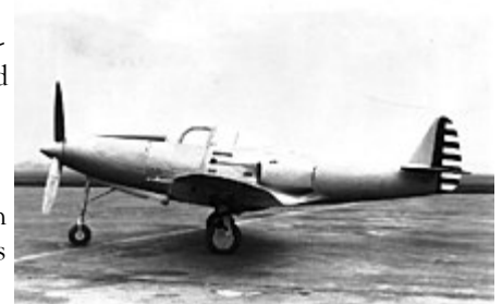
Bell XP-39 showing the position of the supercharger air intake
