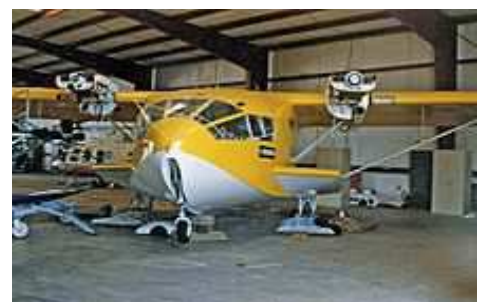
Front view of the Global Explorer showing the deep and wide fuselage, and slot for forward retraction of the nosewheel
