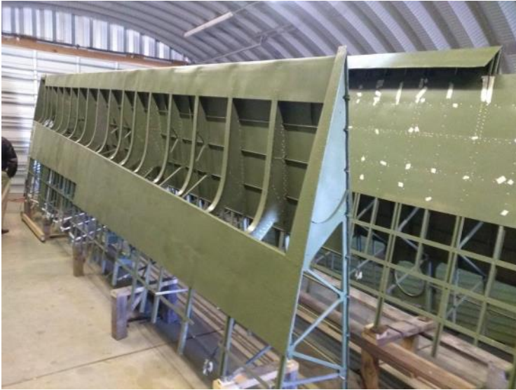
TBM Avenger wings in progress.
