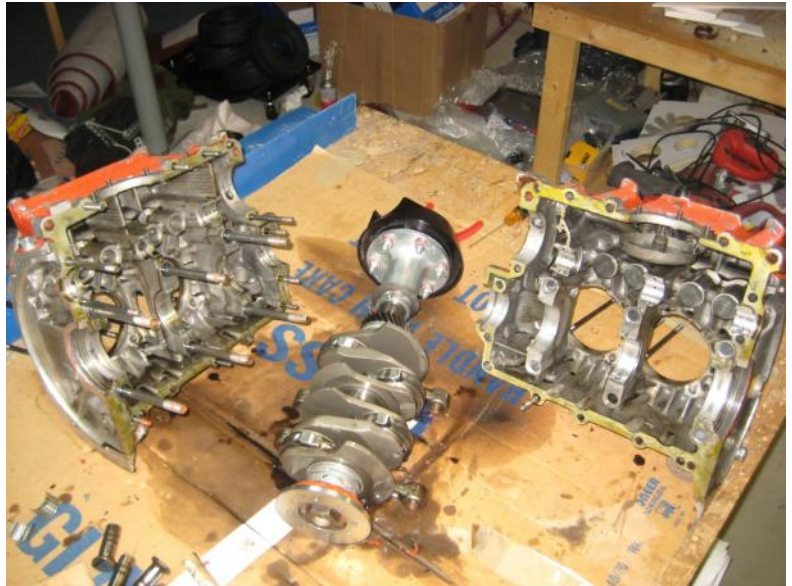
Figure 7: Removing the damaged parts and installing the new bearings and crank.
