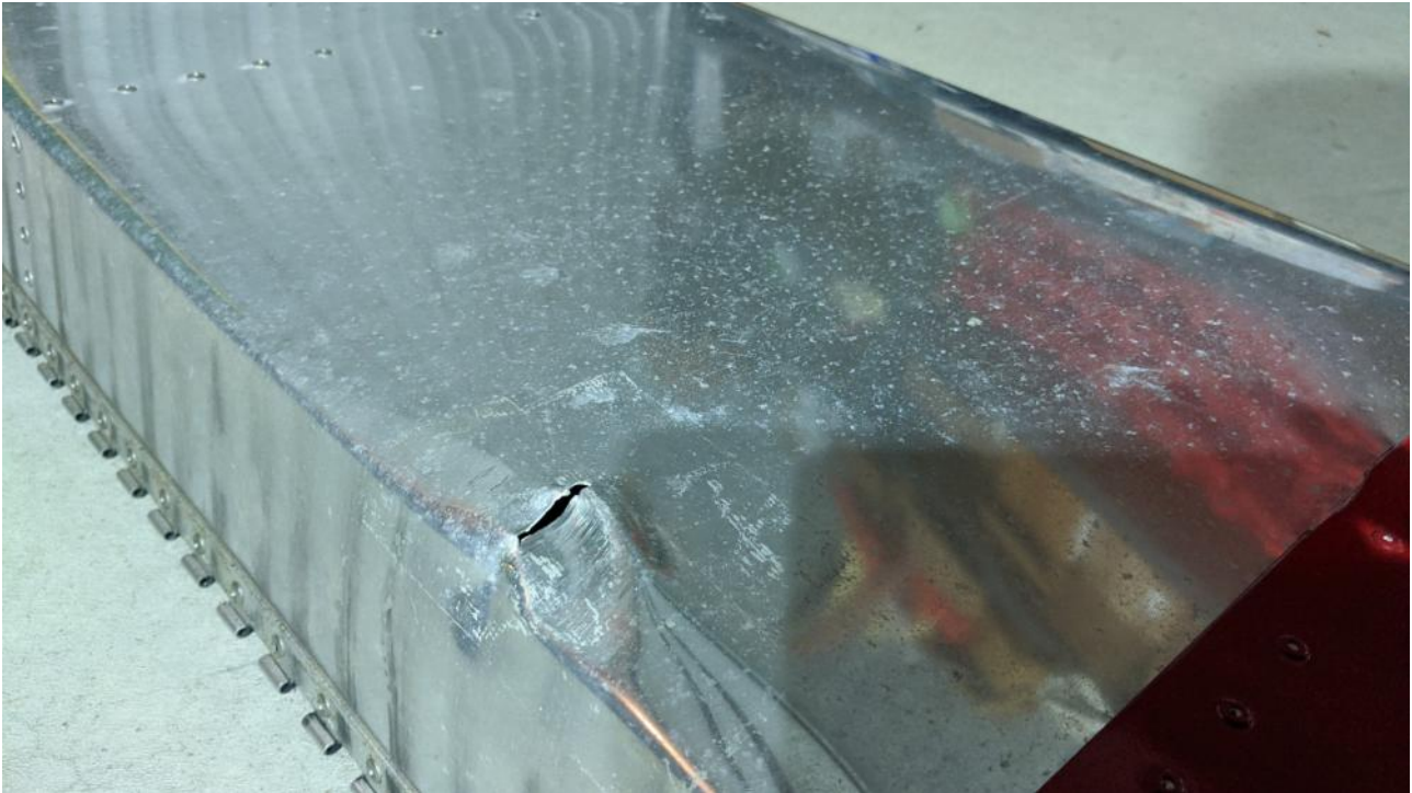
Figure 3: My damaged aileron.
