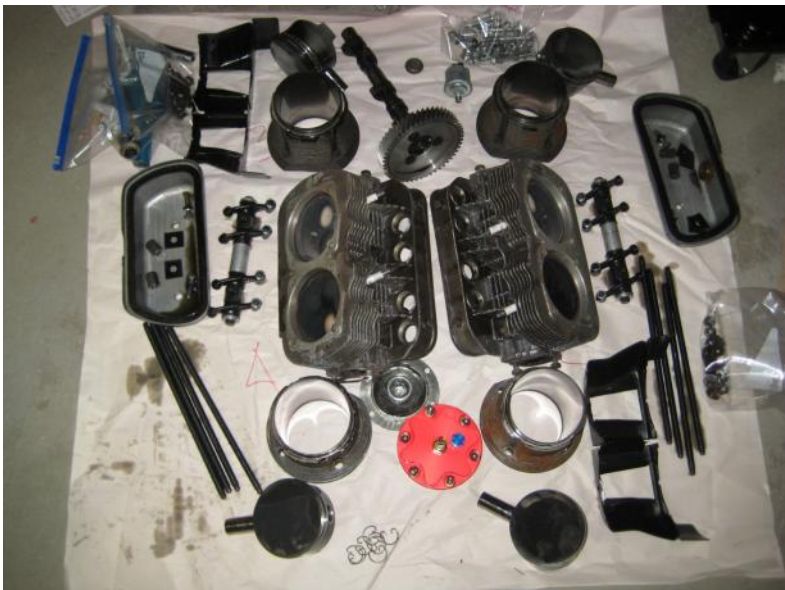
Figure 8: There aren't a lot of parts to an engine as simple as a VW.
