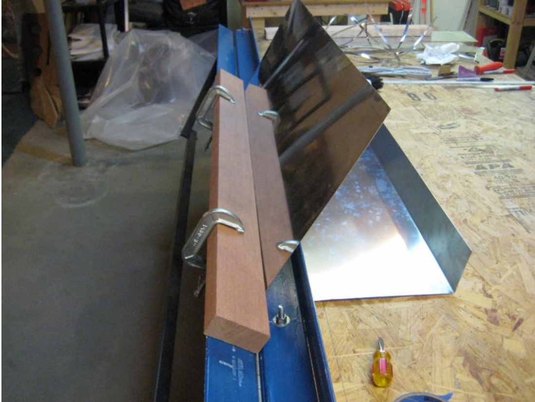
Figure 4: Making a new aileron constructed from plans and raw materials.
