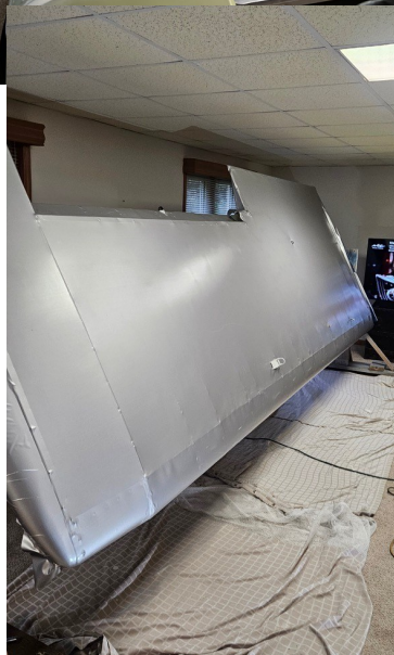
After gluing, the ribs get wide pulled rivets that then will be taped over
