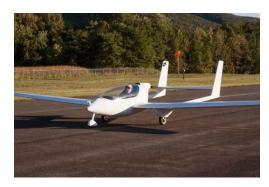
This rear engine motor-glider can stay aloft for about two hours powered only by electricity from the battery packs. Empty weight (without energy source) puts it into the Ultralight Class and coupled with the 20:1 glide ratio, it has very good performance thanks in part to the 37-foot wingspan. The twin tail booms add a box-like structure to the wings-fuselage and provide structural support for the main landing gear.
