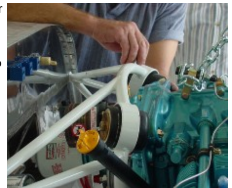
Figure 7. Installing the Second Bolt.
