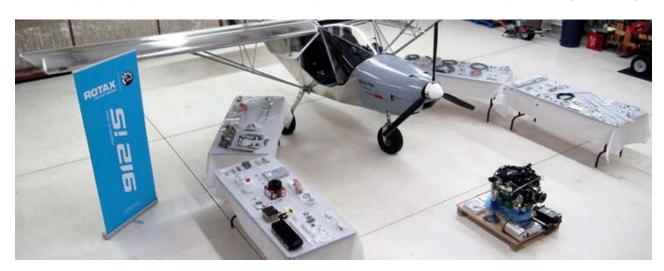
The Rotax 912 iS Sport engine for EAA's One Week Wonder project and its Skytek engine installation kit just prior to shipment to Oshkosh from Skytek. Photo by Skytek Aircraft Services
