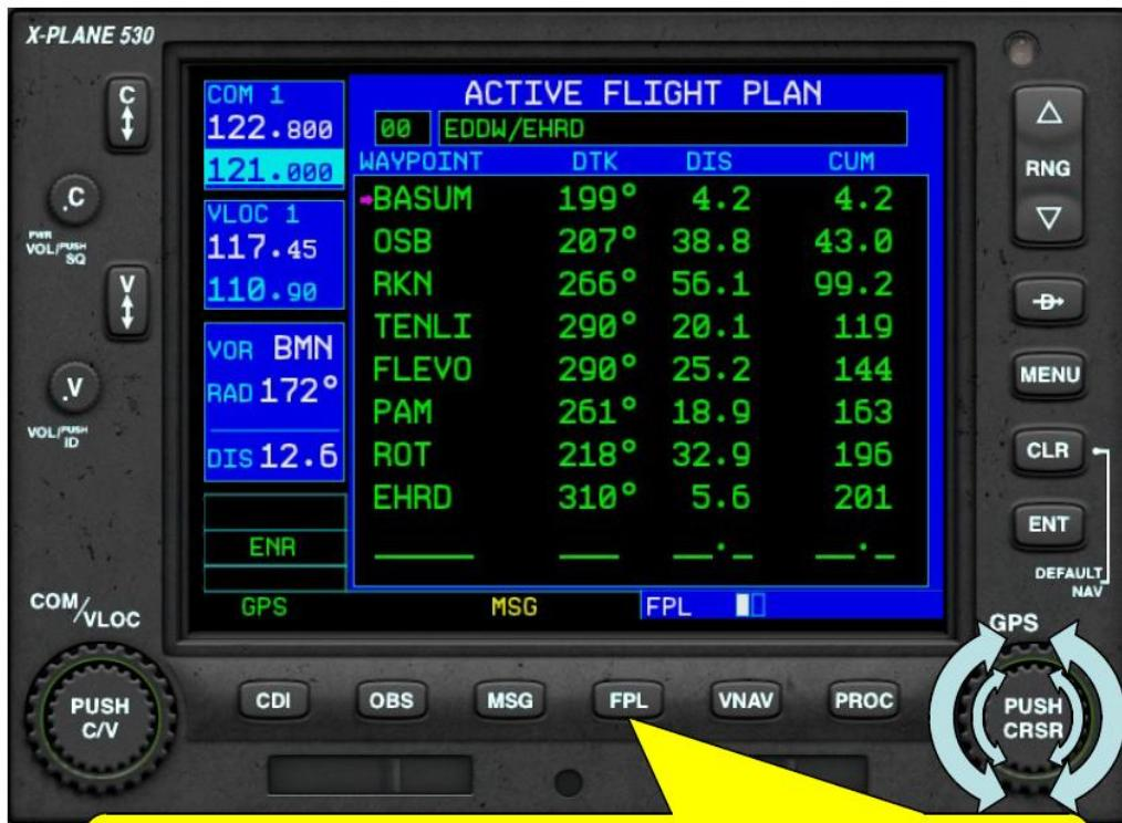
Pressing the **FPL** button toggles the display of this flight plan page showing the waypoints (airports, navaids, intersections, ...) with ID, direct tracking course, distance, cumulated distance, ....
