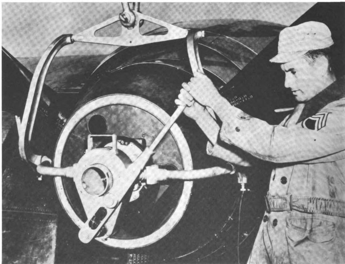
Figure 13.25.—Tightening propeller retaining nut.
