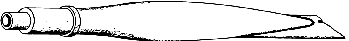
PREFORM BLADE, SEAM WELDED EDGE
