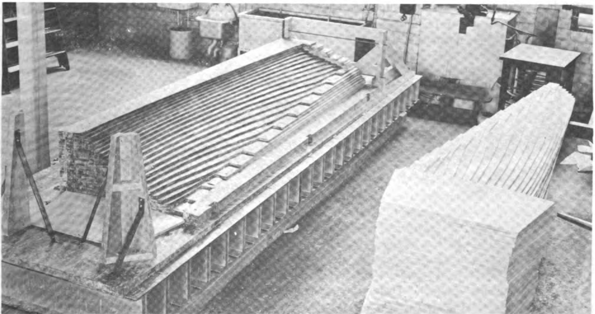
Figure 4.3.—“Stairstep” gluing jig.
