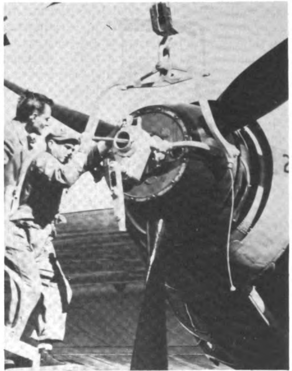
Figure 13.21.—Propeller retaining nut removal.
