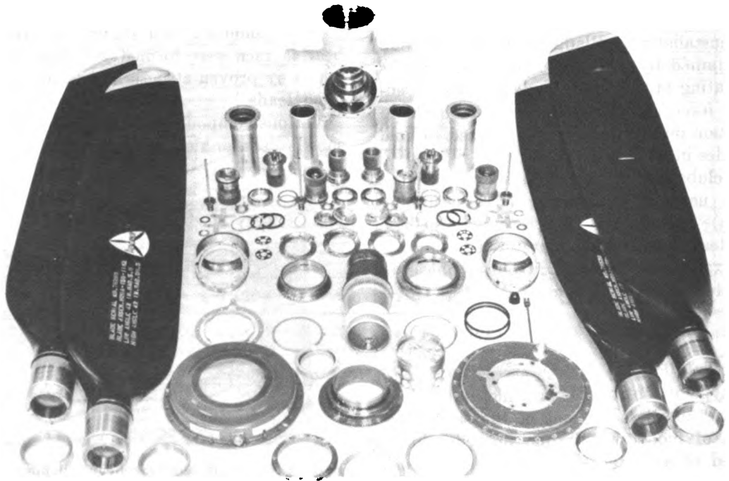
Figure 5.10.—Hydraulic controllable pitch propeller hub, disassembled.
