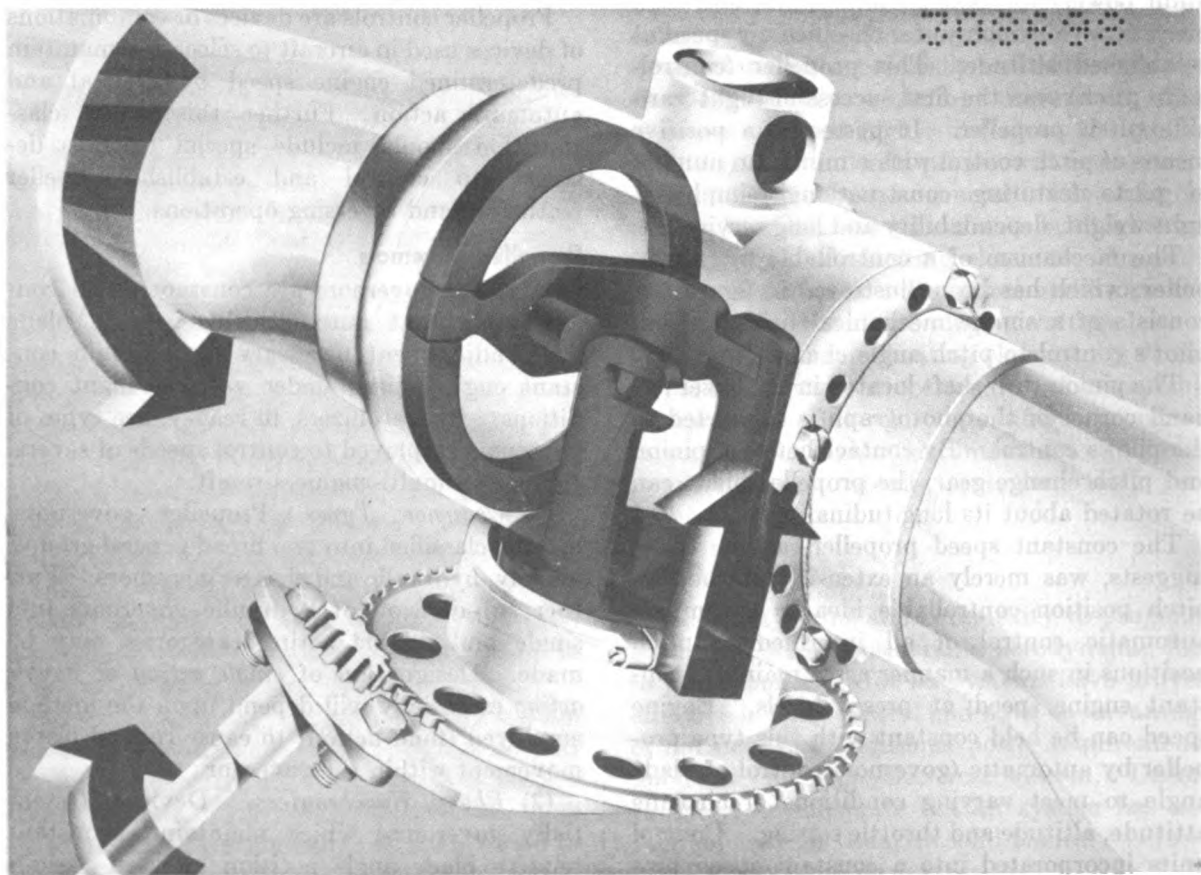
Figure 8.1.—Mechanical pitch control mechanism.
