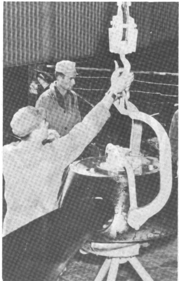
Figure 13.24.—Propeller transfer to vertical spindle.
