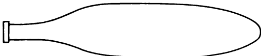
BLADE COMPLETED BY BRAZING CAMBER SHEET TO FORGED AND MACHINED THRUST MEMBER
