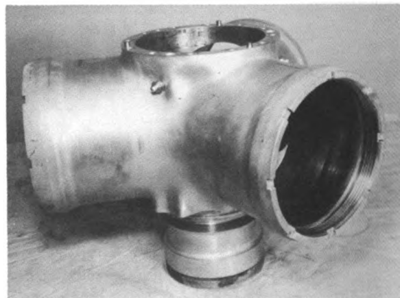
Figure 5.20.—Hub bearing race galling.
