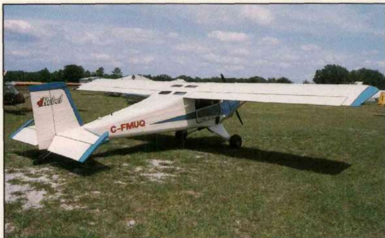
Fabric-covered flaperons extend the full length of the wing. They deflect 18 degrees down and reflex 5 degrees up providing a broad range of flight control.
