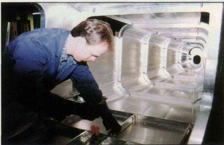
Breaks in the fuselage sides reduce oil canning problems. Fuselage bulkheads are pre-drilled and formed. A false floor turns the plane into a "camper" as well.
