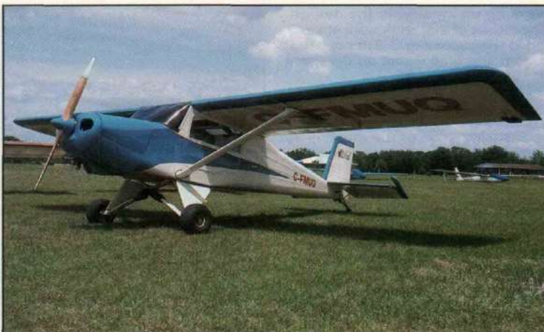
With a 30-foot wingspan, the Rebel exhibits pleasant STOL flight characteristics, stalling at approximately 35 mph with full flaps.
