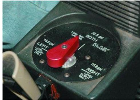
The first takeoff involved an airplane with a worn fuel selector. Pre-takeoff ground operations indicated it wasn't seating properly and allowing full fuel flow to reach the engine, even though the selector's handle was in the proper position. To make it operate consistently and correctly, some greater-than-normal force and some "English" needed to be applied. After fiddling with it and getting a good run-up, I pronounced it good to go. It wasn't.
