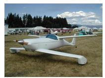
The mystery aircraft to the left is a **Quickie Q2**, a 2-seat version of Rutan's Quickie. This aircraft has a 64-horsepower Volkswagen air-cooled engine. The prototype first flew in 1980. Over 2000 have been built.
