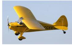
Last month's picture was a **Piper PA-15 Vagabond**. a two-seat high wing aircraft powered by a 65hp Lycoming O-145 engine. The PA-15 Vagabond was Piper's first post-World War II design. The prototype first flew in 1947 with production deliveries in 1948. It utilized much of the same production tooling and components as Piper's famous Cub design. The Vagabond fuselage featured side-by-side seating, rather than Cub's tandem seating.
