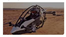
Last month's picture was futuristic EVTOL (electric) aircraft **Jetson One.** Jetson, Inc. describes their aircraft as a Formula One racing car for the sky. Made of lightweight aluminum and carbon fiber, this aircraft weighs in at 121 lbs. empty. Propulsion is from eight propellers governed with a powerful flight computer. Aircraft includes a ballistic parachute.
