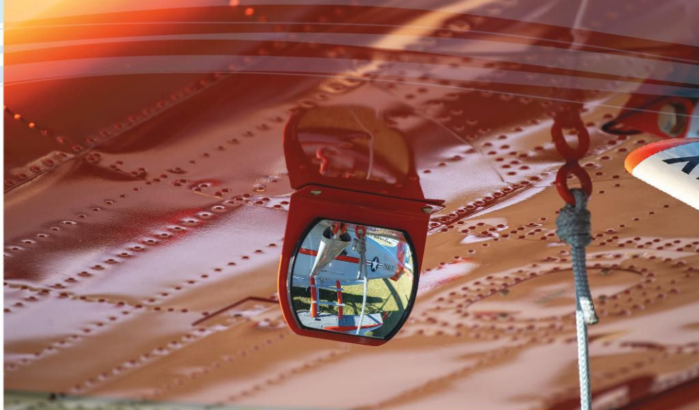
The wing-mounted mirror is the final "gear-up" check before water touchdowns.
