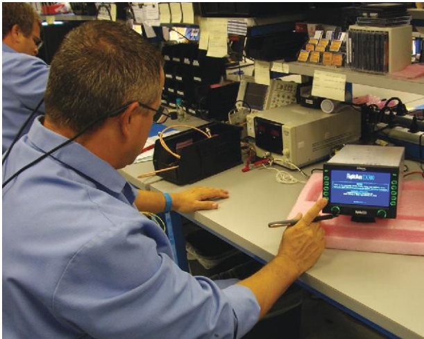
Technician checking out an Avidyne MFD on the bench.
