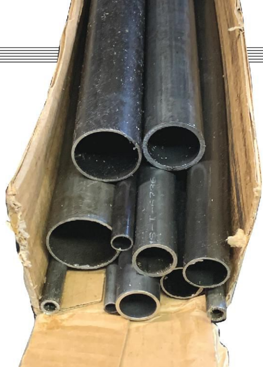
Scrap tubing from various suppliers comes in 18- to 24-inch pieces, and each 10-pound box has tubes ranging from 3/8 inch to 1-1/2 inches for $15. If only one piece solves a future problem, it's well worth the money and takes up little space.
