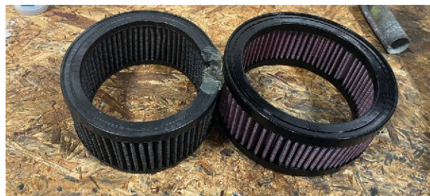
You can clearly see the difference in size between the old filter and the new filter. The old filter was also hard and had caused damage to the bottom of the airbox from vibrating around loose.
