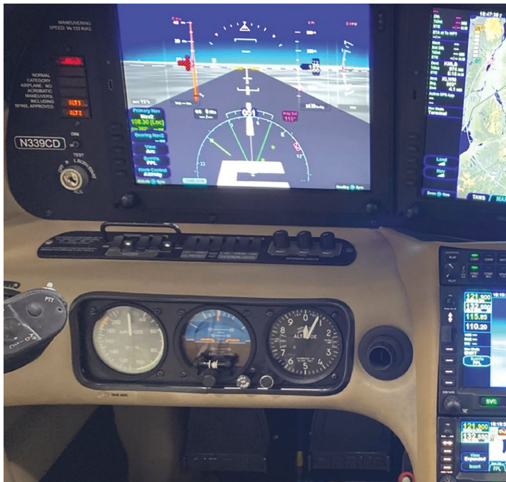
Avidyne’s new Vantage PFD/MFD upgrade for the Cirrus includes 12-inch touchscreen displays with synthetic vision.
