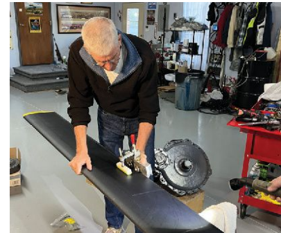
Brad Clark from Vertical Aviation checks the trailing edges of the main blades and performs a delicate static balance of the tail rotor assembly.
