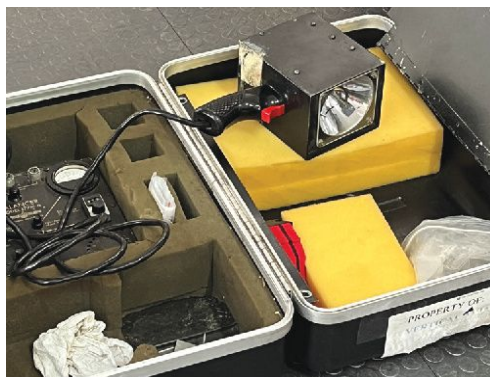
Here you can see the StrobeX light that is used during the blade tracking function of the Chadwick. The strobe light is pointed at the blade tips, on which reflective angles are mounted. The reflective strips each have a stripe in a different direction. Through the use of a magnetic pickup installed on the rotor head, the light is synced to the blades.
