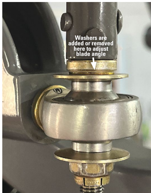
The angle of the blade is adjusted by adding or subtracting washers on the pitch control links.
