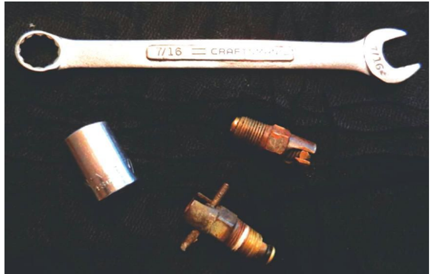
Standard fuel drain (lower left) and one with the crossbar ears cut off (upper right).
