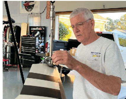
Brad Clark from Vertical Aviation checks the trailing edges of the main blades and performs a delicate static balance of the tail rotor assembly.
