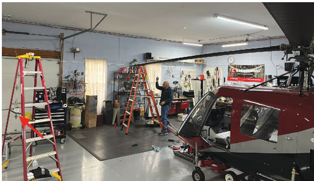
By using a simple pulley and weight system, I could time the blade travel across the full range of the blade dampener. They all need to be close to each other in timing.
