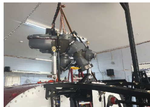
An A-frame gantry crane makes removal and installation of the rotor head and transmission easily done by one person.
