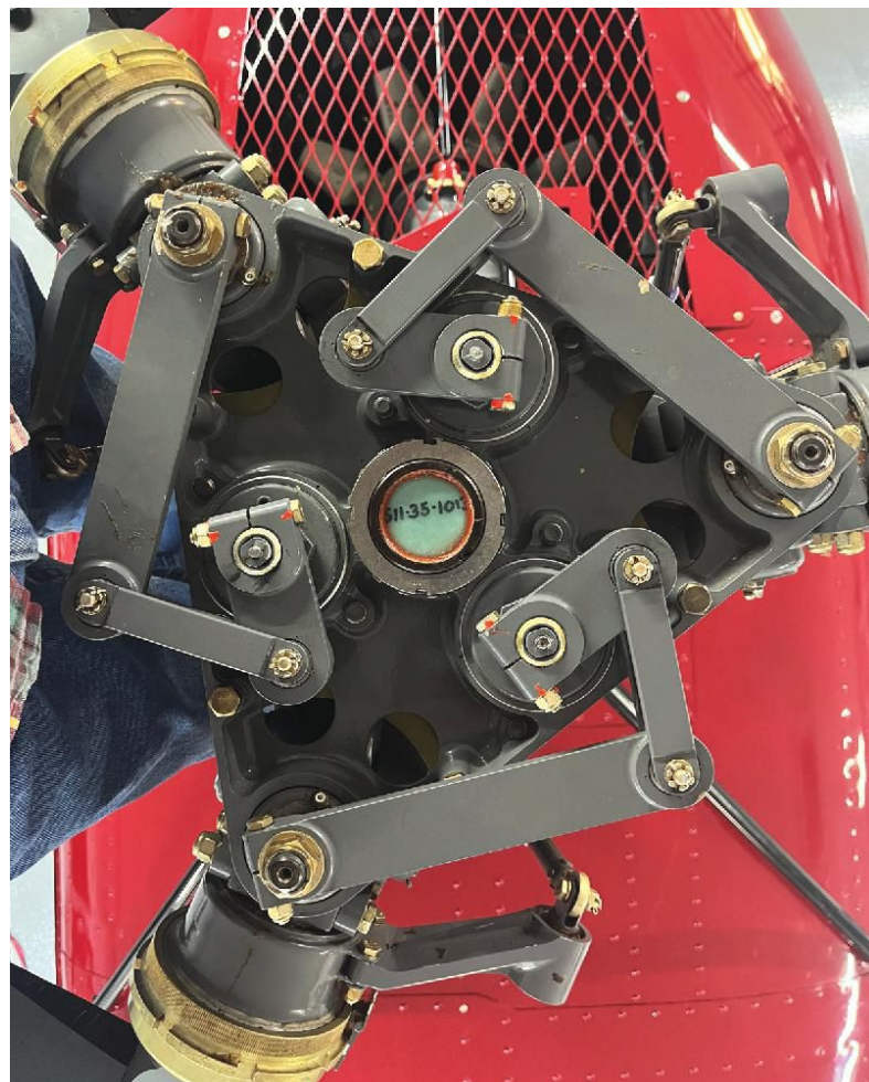
In these pictures, you can see the pitch control links and blade dampeners installed on the rotor head.
