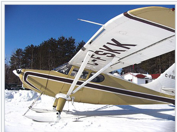
Partial-span leading-edge slot in the wing of a Stinson 108-3
