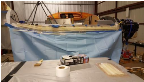
Fiberglass cover for BRS parachute rear straps
