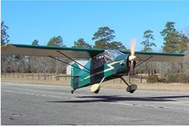
It is a Zippy Sport LSA designed by Ed Fisher and marketed by Green Sky Aviation. The Zippy Sport is a single-seat, high-wing monoplane powered by a 50 hp (37 kW) Rotax 503 piston engine. Other engines have been fitted, including VW. Of mixed construction, it has a welded 4130
