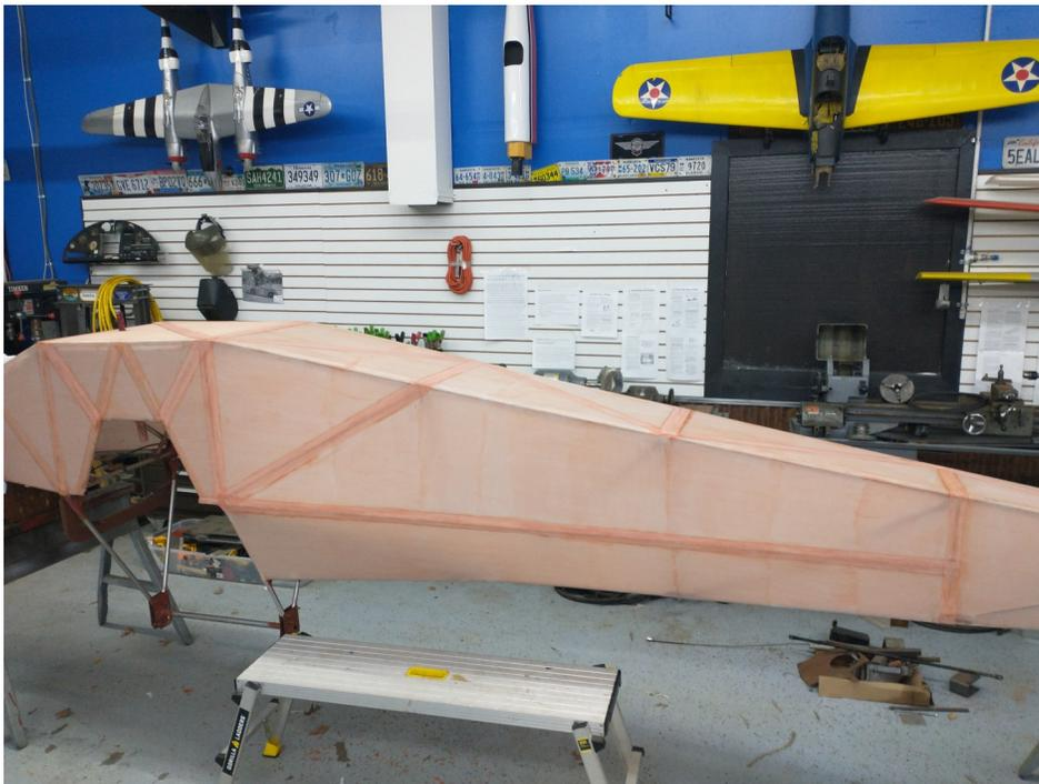
Work continued through November applying reinforcement tape to the fuselage. These are the darker-colored strips seen in the photos. This is a tedious process required wherever the fabric contacts the 'skeleton'. There are plenty more sections to complete including all the pieces that comprise the tail.
