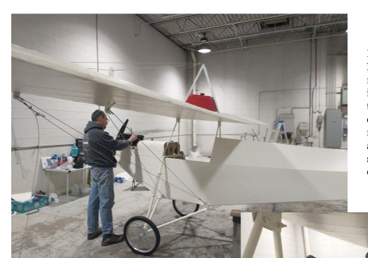
During our next meeting on November 23rd, we experimented with different hardware items to determine the best way to attach the 'downward-force' cables . We determined the need for additional turnbuckles and fasteners to make the design stronger as well as easy to dis-assemble.
