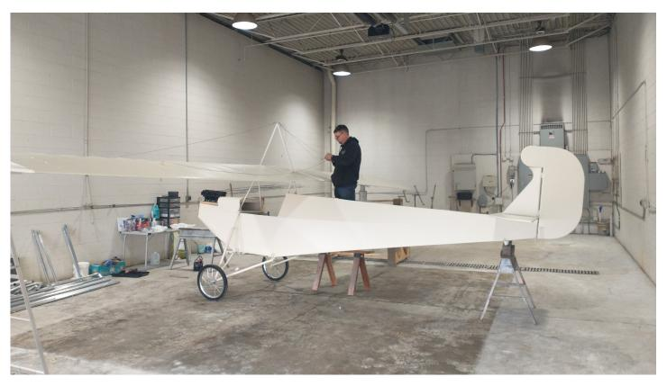
Once the wings were attached to the fuselage, the next step was to string steel cable to hold them up. And yes...that red container is the gasoline tank.
