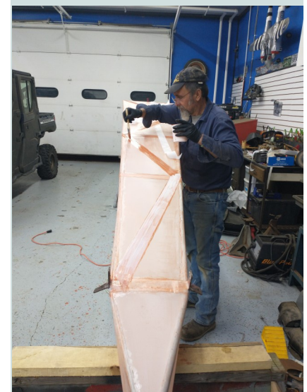
November 3: Joe applying finishing tapes with PolyBrush.
