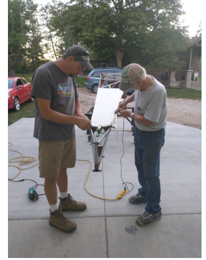
Work underway to prep the fuselage, flip the frame on its “back” and lay the first section of fabric.
