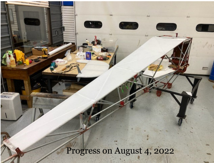
Work underway to prep the fuselage, flip the frame on its “back” and lay the first section of fabric.
