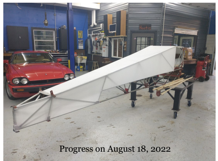
Work underway to prep the fuselage, flip the frame on its “back” and lay the first section of fabric.
