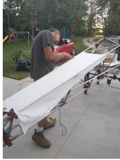
Work underway to prep the fuselage, flip the frame on its “back” and lay the first section of fabric.
