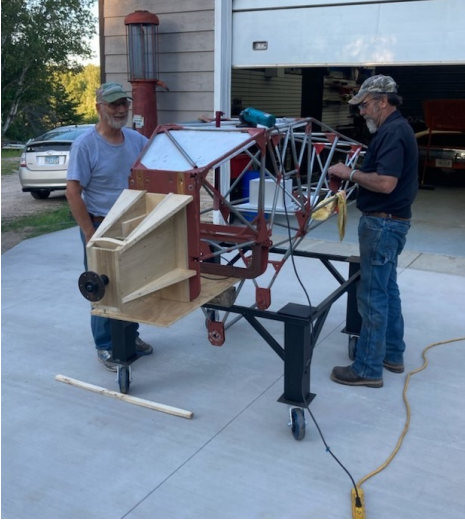
Work underway to prep the fuselage, flip the frame on its “back” and lay the first section of fabric.
