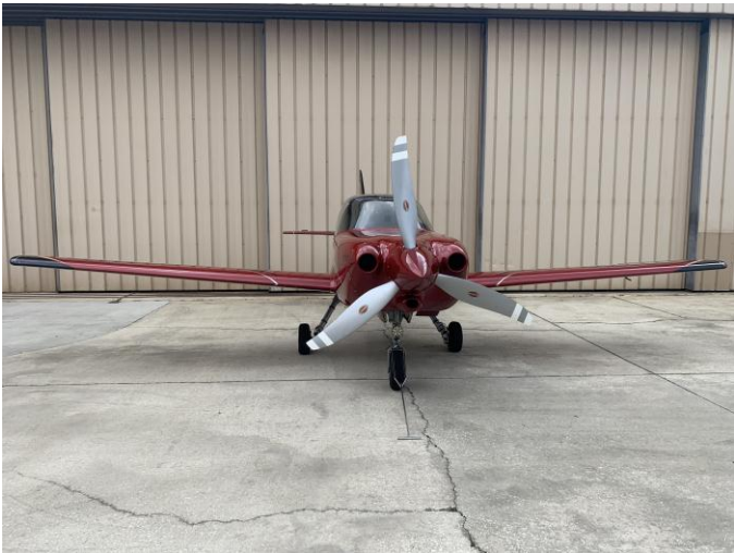
There was an interesting display of Swearingen SX300 aircraft. Designed by Ed Swearingen (who created the prototype of the Piper PA-30 Twin Comanche). These little marvels claim to be the fastest all metal single engine experimental classified aircraft ever built. It has an IO540 engine and at 65% HP it cruises at 210-220kts. Stall speed 71-91kts. To achieve the aerodynamics the aircraft comes with retractable landing gear. The aircraft has a poor safety record with numerous fatalities and collapsed gear on landing. But these ones look great! One was for sale for $225K USD with 1170 on the hobbs.
