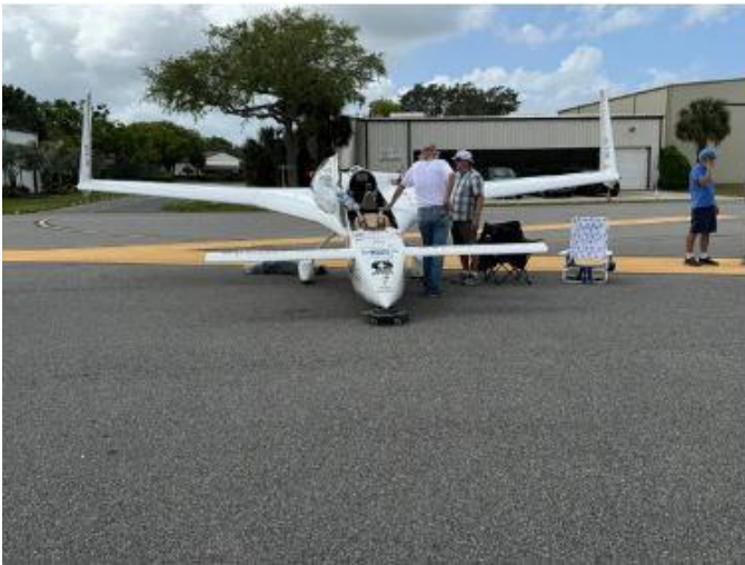
There was an interesting display of Swearingen SX300 aircraft. Designed by Ed Swearingen (who created the prototype of the Piper PA-30 Twin Comanche). These little marvels claim to be the fastest all metal single engine experimental classified aircraft ever built. It has an IO540 engine and at 65% HP it cruises at 210-220kts. Stall speed 71-91kts. To achieve the aerodynamics the aircraft comes with retractable landing gear. The aircraft has a poor safety record with numerous fatalities and collapsed gear on landing. But these ones look great! One was for sale for $225K USD with 1170 on the hobbs.
