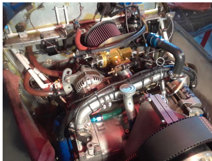
Rotec TBI Installed
