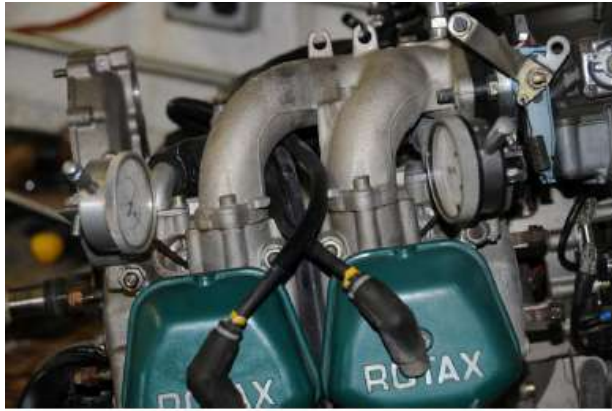
Checking cylinders 2 & 4, top dead against bottom dead center
