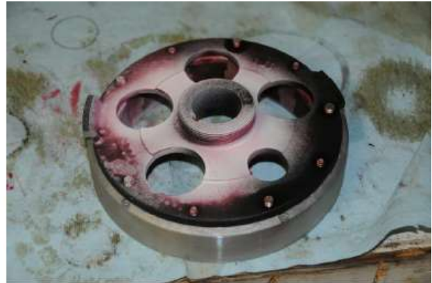
Die penetrant crack detection - flywheel
