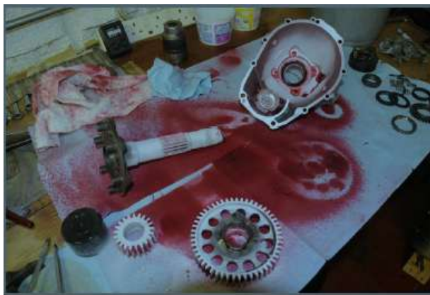
Die penetrant crack detection - gearbox parts
