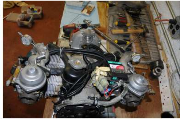
Checking cylinders 1 & 2, both at top dead centre
