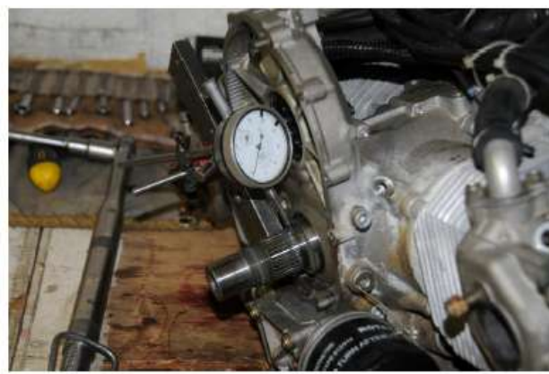
Crankshaft PTO end out of true check
