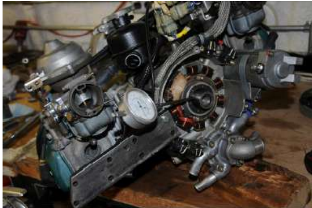
Checking PTO end crankshaft out of true
