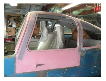
Installing the panel was rewarding. Designing the locations of everything so that they felt comfortable and where the wiring would be placed. I did not fabricate a harness for everything, I ran each wire by its self.
