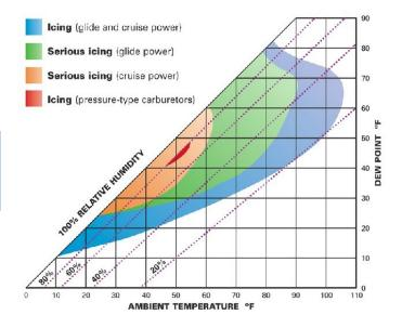
The carburetor was operating in the upper right of the above chart. My only other experience with carburetor ice was in my 1946 BC12D Taylorcraft at 9,500 feet when the engine started loosing RPM. Carburetor heat was pulled, it ran really rough, and then recovered. The rest of that flight was with carburetor heat on.
