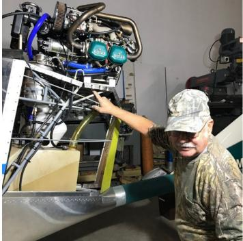
Above is the Titan Tornado II undergoing repair of the engine mount, longeron members, and sheet metal. Steve fabricated a replacement engine mounting base support which is better than the original. Sheet metal was formed to replace existing panels and fabric in need of repair.
