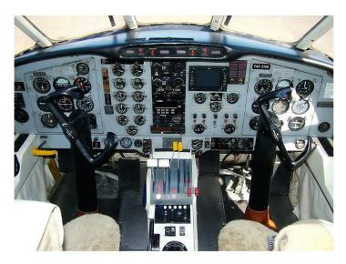
Bandeirante flight deck with steam gauges and a weather radar display screen (Wikipedia photo)
