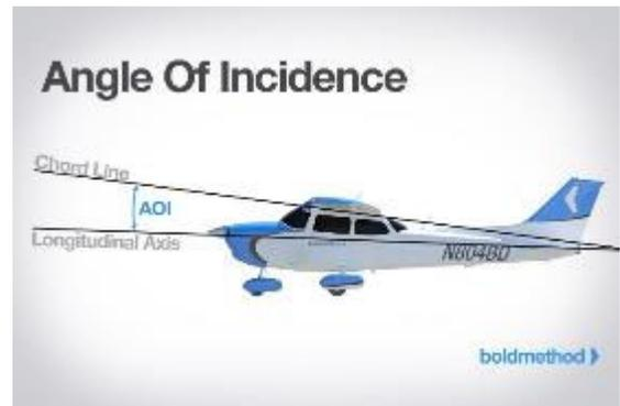
VIII. **Wing Washout** - Washout is a change in an airfoil's angle of incidence, measured from the root to the tip. If you look closely at a wing with washout, you'll see that it twists from the root to the tip, with the root having a higher angle of incidence than the tip.
