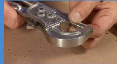
**Flush Riveting with Hand Squeezer**
