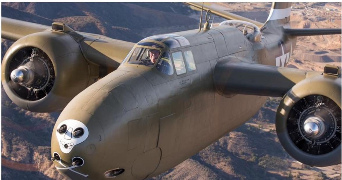
Lewis' Havoc was built in 1943 as an A-20G, is powered by two 1,700-hp Wright R-2600s, armed with seven 7.7mm (.303 caliber) machine guns (six Brownings, one Vickers) and could carry a bomb load of 4,000 pounds. The airplane was previously owned by the Lone Star Flight Museum, but has since been fully restored to its original, stock military configuration. AirVenture Oshkosh 2016 is expected to be the A-20's first official public display since the restoration.
