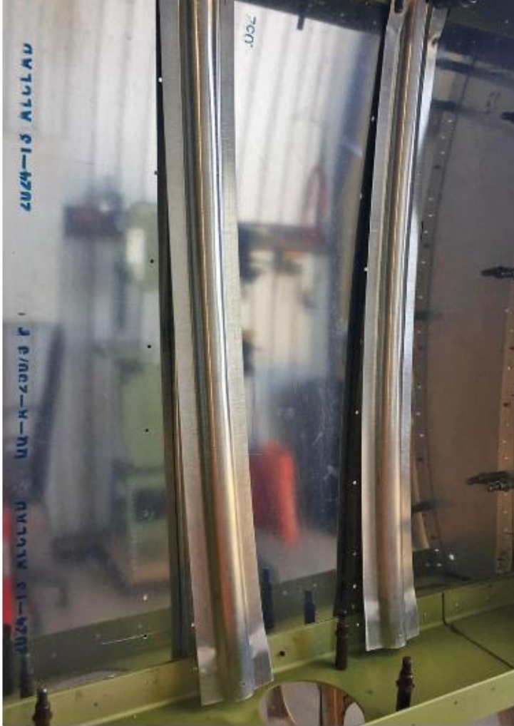
The problem: GlaStar hat sections have to be drilled through from the outer wing skin (left), but there's no way to hold them in place on the inside of the skin. Here's the final fixture (right) ready to be used.
