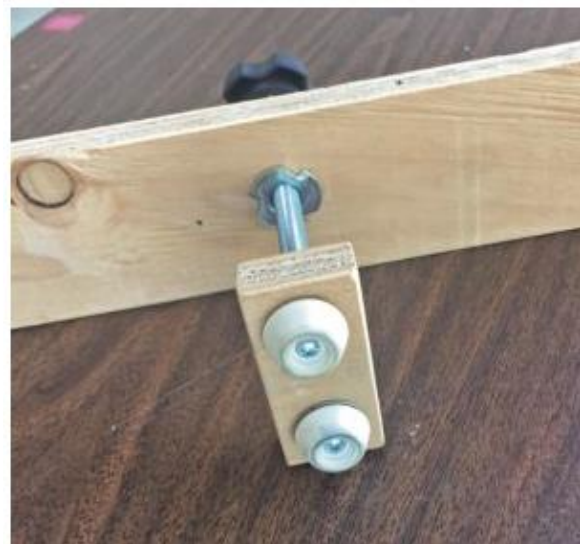
Bumpers hold the hat section in place without marring the surface.
