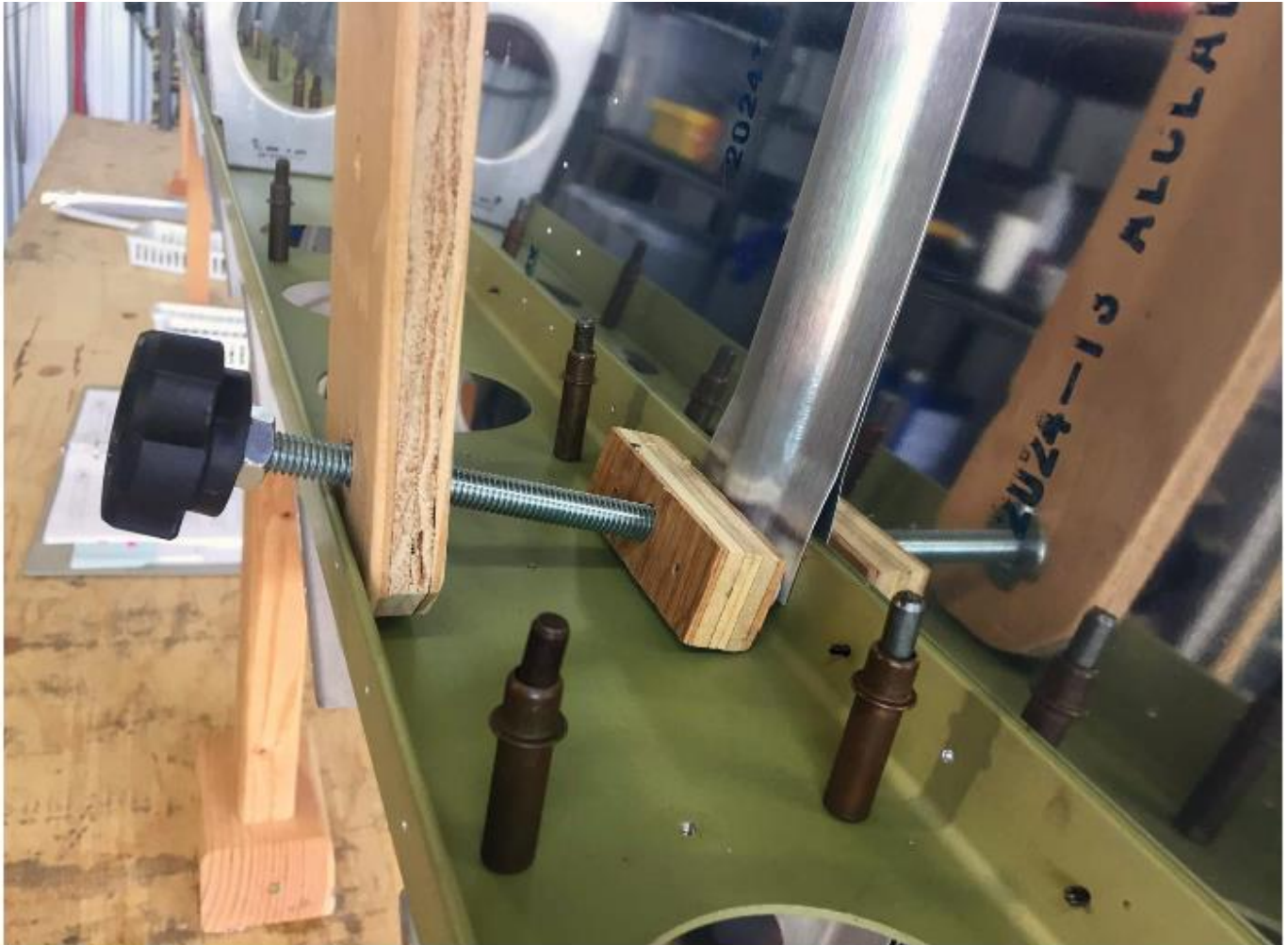
At the outer edges of the hat section, the "third-hand" jig rests inside the spar channel. Note the angles needed to place the foot in the correct spot.
