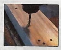
9. Drilling out flush rivets uses the same process. After center-punching the factory head, start the drill slowly and drill down just until you reach the shank.
