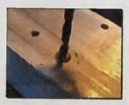
3. Start the drill with a few short, slow pulls of the trigger; the idea is to center the bit in the dimple before starting to really drill. Once you start drilling, make sure you actively steer the bit into the center of the rivet head.
