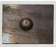
1. The factory head on this universal-head rivet is fine, but the shop head wasn't up to spec, so out it comes. Note the dimple in the center of the head; this can be enough for experienced builders to use to center their drill bit.
