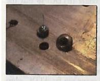
8. If you do a clean job removing the rivet, you will be able to keep the shop and factory heads as souvenirs. (Unfortunately, even the best builders have quite a collection of drilled-out rivets, so they won't fetch much money on the collector's circuit.)
