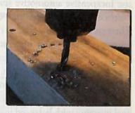
11. If you have perfectly centered the drill bit, the remains of the head might just climb the bit itself. In either case, pop the remains of the shank and shop head out the back side and get on with your build.
