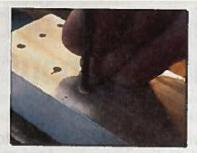
5. Use the back side of a jobber drill bit (the same size as your rivet) inserted into the hole to break off the head.
