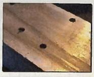
7. The tool may then be used to push the tail of the rivet out the other side, leaving a clean hole for your next riveting attempt.
