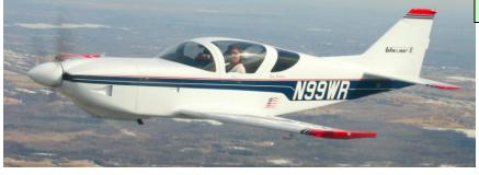
The fiberglass construction gives a smooth, fast, and efficient finish. The kit is supplied close to the 51% rule. The factory builds the more difficult parts, such as the spars, machined control components, fuselage halves, and landing gear.
