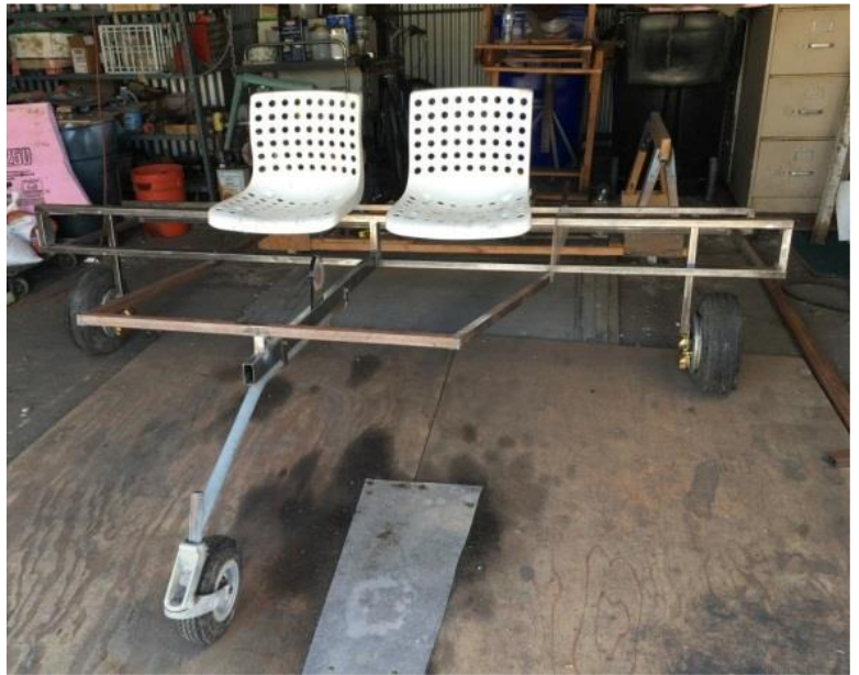
Nose wheel assembly installed.
