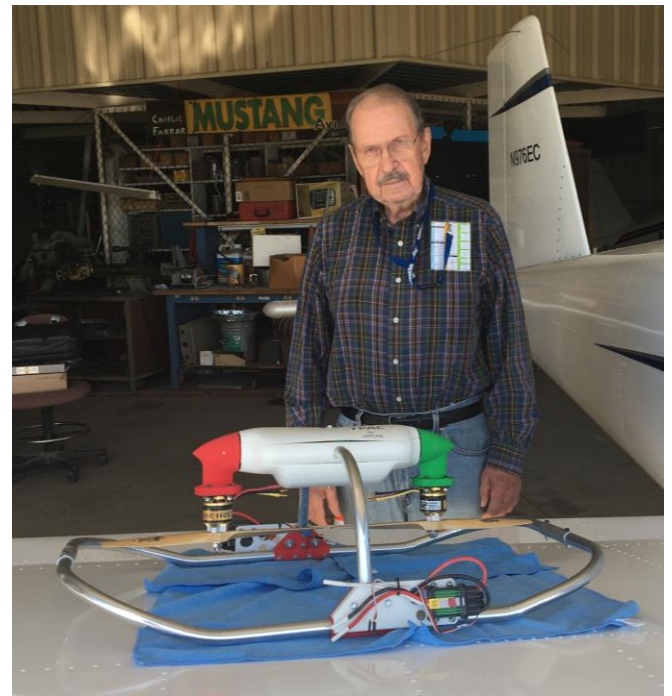
Gert Lundgren shows off his prototype two-rotor drone. The rotor heads tilt to provide directional control.
