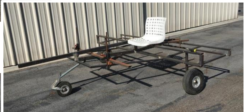
Keel started for making a bed mount for the engine.
