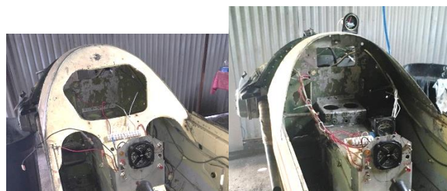
Before and After. The cockpit front bulkhead, shown in place on the left, made it impossible for Ryan to make a template for his new header tank. Removing the bulkhead (right) gives room to fit the new header tank. The quad engine instrument is visible on its temporary mount in the center of both photos.
