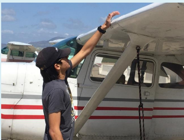
Ryan checks the stall warning system for insects during a pre-flight inspection.
