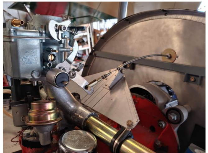
Throttle linkage on Gene Hubbard’s Nieuport. It’s a stock VW carburetor, but needs an extension arm on the throttle to get the angle of the cable right.
