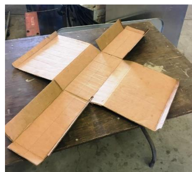
Cardboard mockup for Ryan's new four-gallon header tank. Cardboard is easy to work and cheap—Make your mistakes here.
