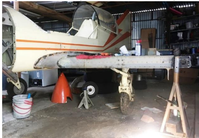
Preparation for gear retract test. With the plane on jackstands, Ryan cycles the landing gear
