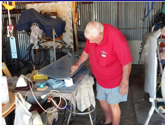
Jimmy Kennedy wet sands the seam tape on his Nieuport elevator. 10/21
