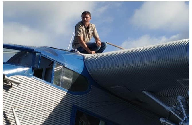
Trevor fuels the Tri-Motor between flights. It uses about 60 gallons per hour.
