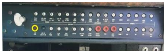
Color-coded circuit breaker collars help identify critical circuits in the event of an emergency.
