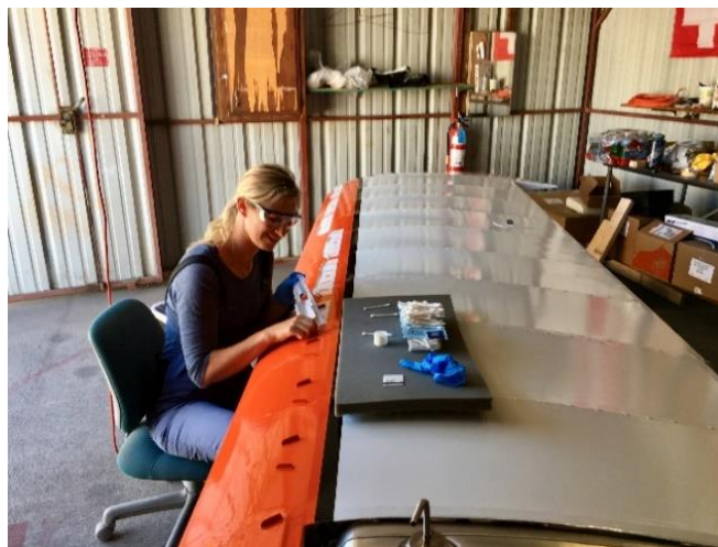
Jackie installs vortex generators on the plane, now named "Pocahontas."
