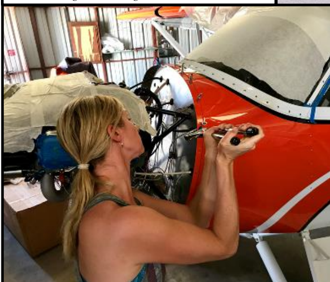
Jackie squeezes some rivets. It looks like she's installing nutplates for the engine cowling.
