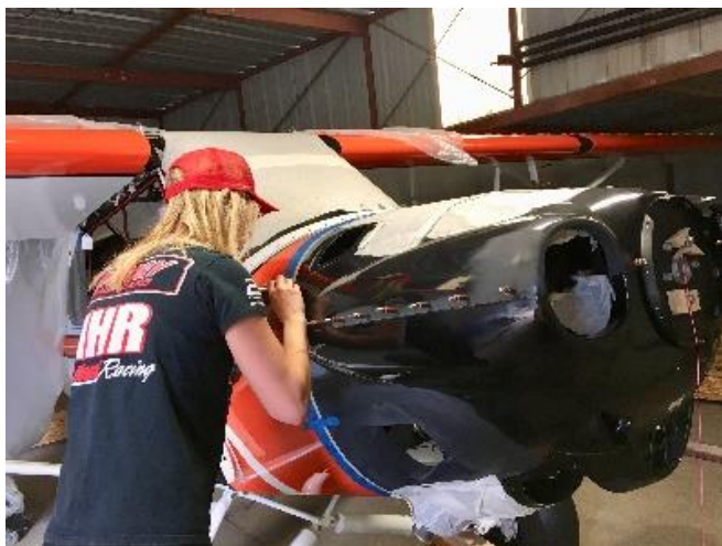
Jackie marks the engine cowl for trimming and mounting
