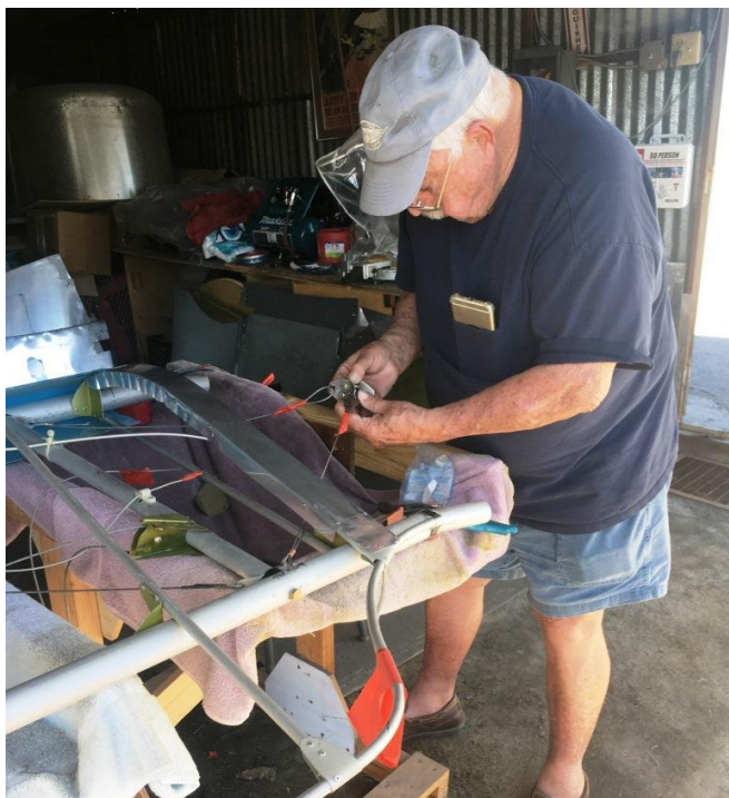
Jimmy Kennedy works on root rib bracing in preparation for covering his Nieuport 11 wing.
