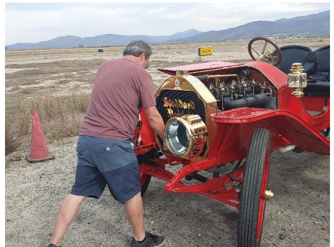
Dave Eby demonstrates hand cranking technique to start his Stoddard Dayton. He also demonstrated a much less athletic technique using the spark advance
