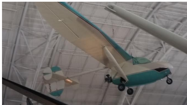
Bowlus/Nelson Dragonfly. Probably the most practical of the three. They built seven in 1947 to promote the Nelson 25hp engine. It's been described as an "underpowered sailplane." Climb was 235 fpm at sea level.
