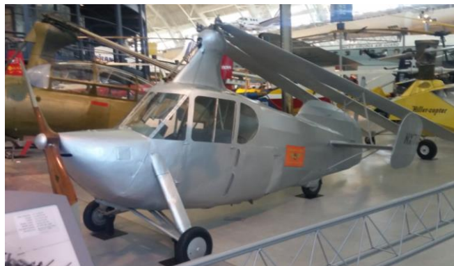
Here's an interesting concept: the Autogiro Company of America AC-35. It's a flying car from 1935. You land, fold back the rotor, and drive away powered by the tailwheel and steering with the front wheels. 5/24
