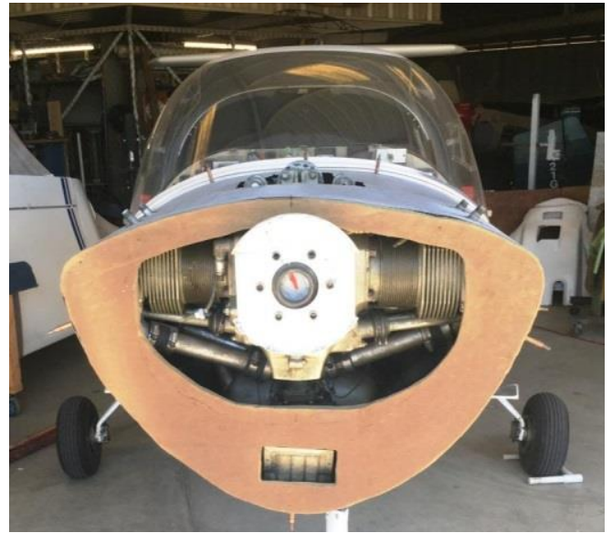
First try at a cardboard pattern for the nose bowl. Close but not there yet
