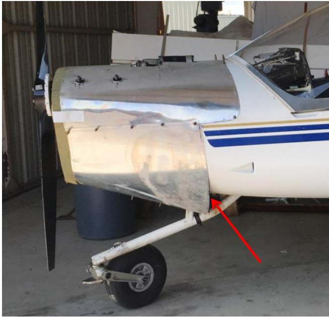
First attempt at a lower cowling. It fits, but the large exhaust area for cooling air (red arrow) makes it look clunky.
