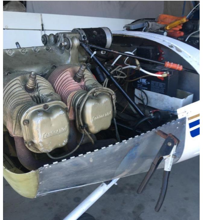
Piano hinge installed
