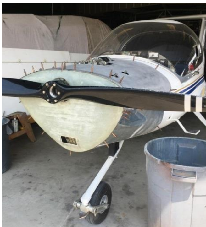
Second nose bowl clecoed in place. More layers of fiberglass and this time it didn't warp.
