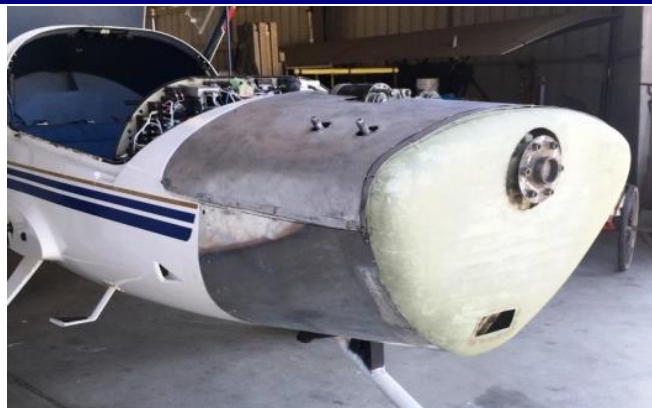
Uncut nose bowl riveted in place
