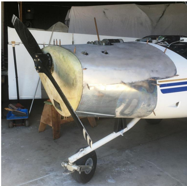
Next try was a form-fitting lower cowl. Much sleeker look and we’ll find another way to let the cooling air out.
