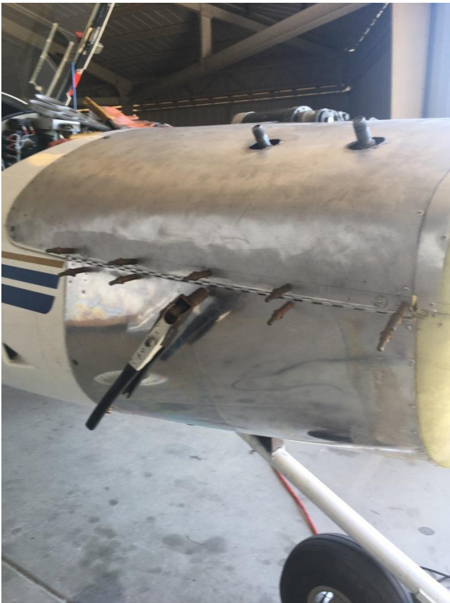
Piano hinge clecoed in place before riveting
