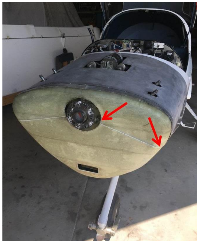
Time to cut the nose bowl apart. The cut line (red arrows) extends from the center hole to where the top upper and lower aluminum pieces join.
