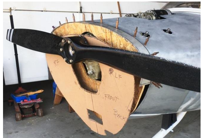
The next try at a cardboard pattern worked. Then Ryan transferred the pattern to a plywood plug for stiffness.
