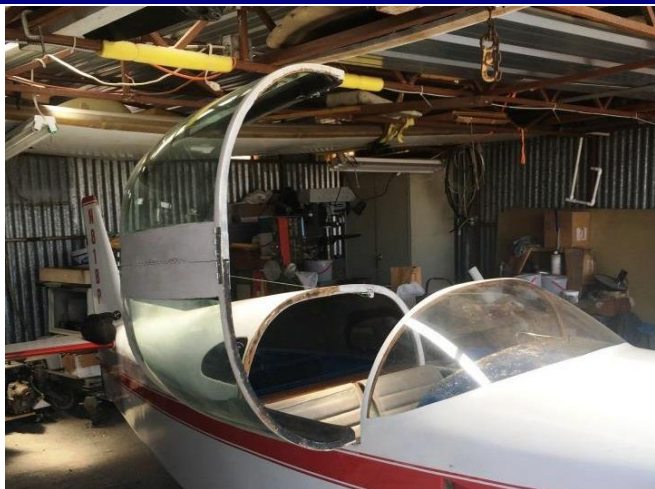
Ryan's KR-2 in his hangar. The full-opening canopy makes it a lot easier to get in and out, especially for the right-seat passenger.
