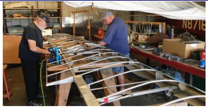
Chuck Stiles and Jimmy Kennedy prepare the top wing on Jimmy's Nieuport for covering
