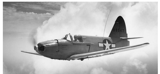
Culver TD2C-1—the military drone version of the Cadet flown by the Navy. They flew it by radio control when people were shooting at it. This is a US Government photo probably taken around 1945. As a drone, the plane would have been painted all orange.
